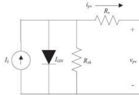
Fig.4 Equivalent circuit diagram of the PV cell
