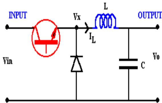
Fig 5 Buck Converter
