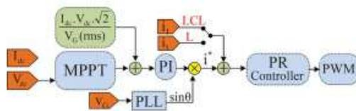
Fig8: Basic control of a single-phase PV.
