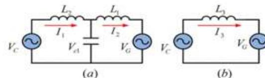
Fig7: Simplified PV model with different filters. (a) LCL filter. (b) L filter.
