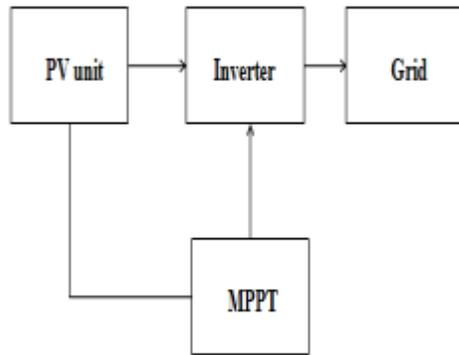
Fig. 3 Schematic diagram of PV system
