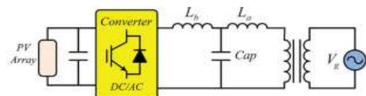
Fig. 2. Basic configuration of PV system.
