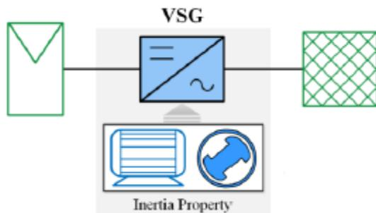
Fig. 1. Basic concept of a VSG.
