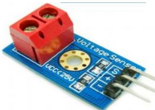
Fig.6. Voltage Sensor
