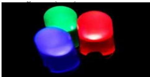
Fig.8. Red, Pure Green and Blue Leds of the 5mm Diffused Type
