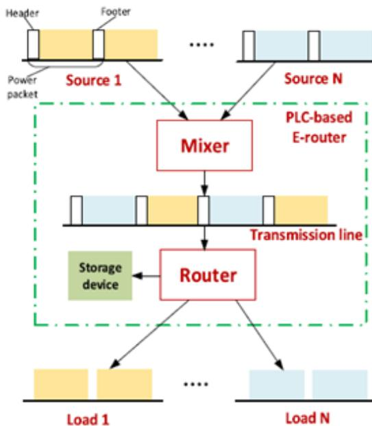
Fig. 4. PLC based energy router
