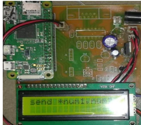
Fig 5: Send the Registered mobile no and users mobile number
