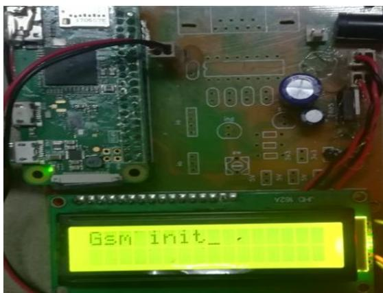
Fig 4: GSM Module getting Initialized
