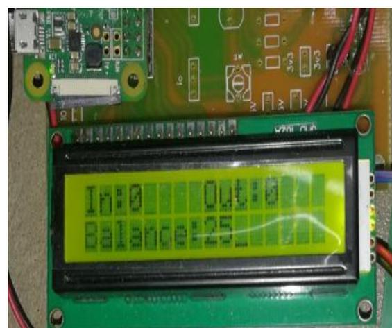
Fig7: LCD displaying Balance amount
