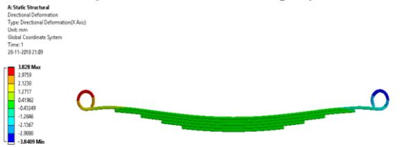
Figure 8 Directional deformations in E Glass/Epoxy
